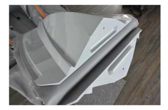
The underwater shape (of the solid glassfibre hull) widens and flattens in the run aft, to make a nice steady planing surface. This is also VERY efficient: F-RIBs are unusually fast compared to other RIBs, size for size and hp for hp.
